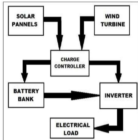
Fig. Block diagram of Hybrid energy generation system
