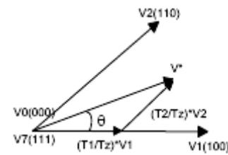
Fig 9.1 Determination of Switching times
