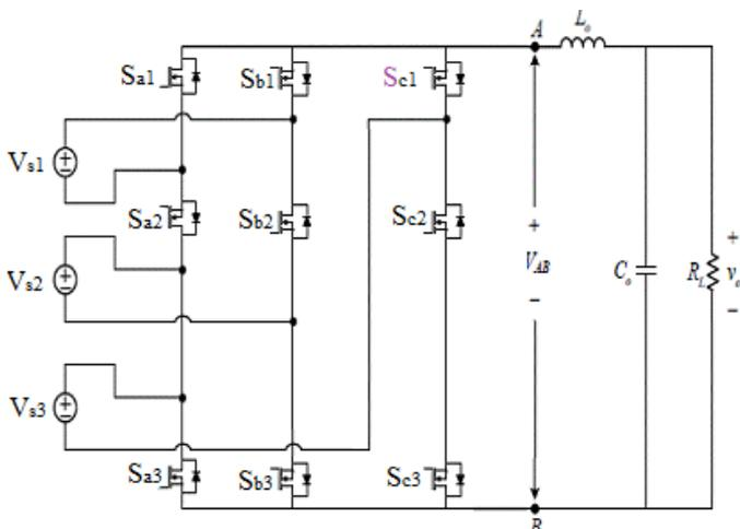
Fig.3. Basic Seven-level inverter circuitry.
