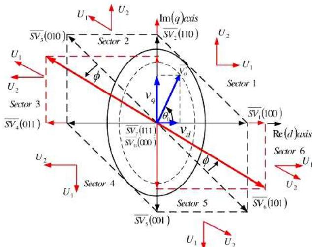
Fig 9.4. SVM Vector Diagram for New Switching Converter
