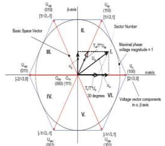
Fig.9. Inverter output voltage space vector
