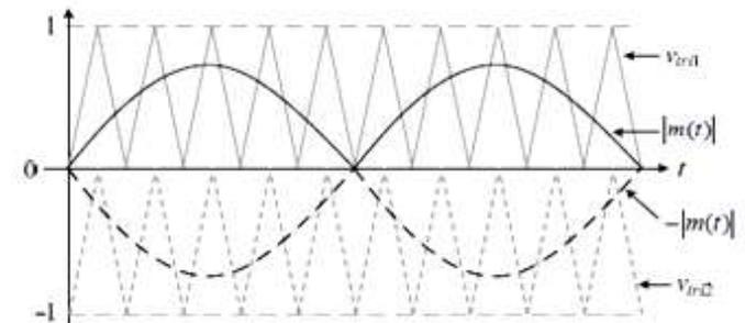
Fig.4 Modulation strategy: carrier/reference signals
