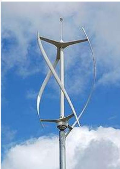
With a vertical axis, the generator and other primary components can be placed near the ground, so the tower does not need to support it, also makes maintenance easier. The main drawback of a VAWT generally create drag when rotating into the wind.
