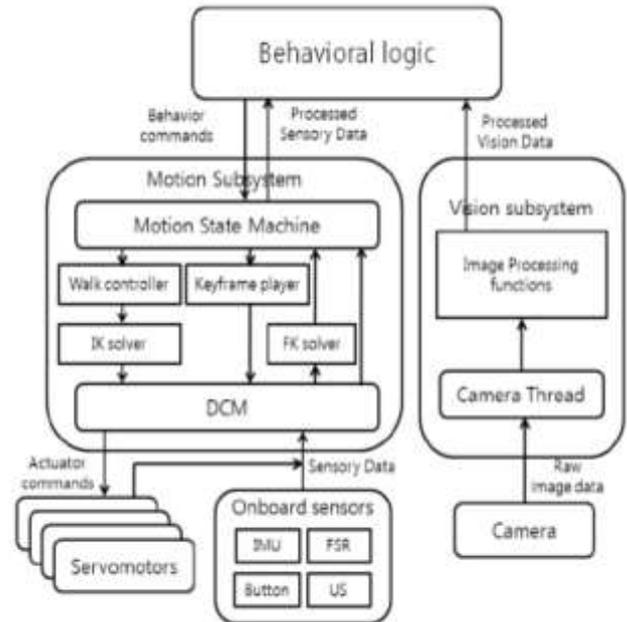
Fig. 2. Block Diagram of the Software Architecture
