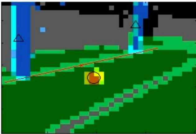
Fig. 3. Results of Image Processing, where the ball is circled
