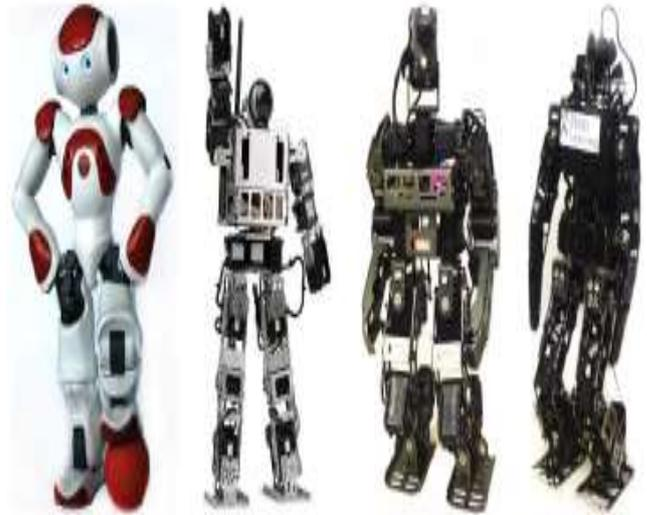
Fig. 1. Various supported humanoid robotic platforms, from left: Aldabaran Nao, MiniHUBO, DARwIn LC, DARwIn HP
