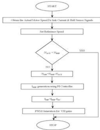
FIG 10 Flow chart for Speed Controller
