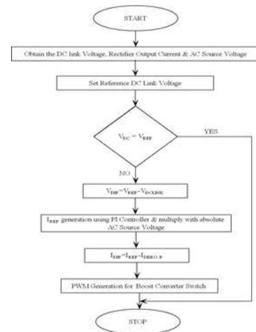
FIG 9 Control Flow chart for Voltage Controller
