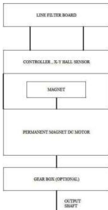
**FIG. 2 Schematic block diagram of an integrated motor controller constructed in accordance with the principles of the projected research**
