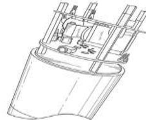
**FIG. 3 Perspective view of the integrated motor and controller in accordance with the present invention with the housing for the controller removed**
