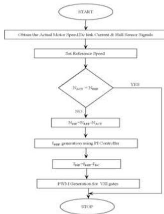
FIG 10 Flow chart for Speed Controller
