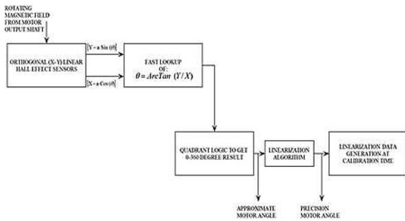
FIG 7 Diagram illustrating the termination of the motor angle from the Hall Effect Sensor data
