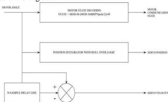
FIG 8 Diagram illustrating extraction of the motor state servo position and servo velocity from motor angle
