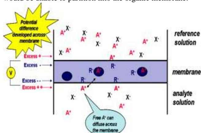
Figure 3. Development of a potential at an ISE.
