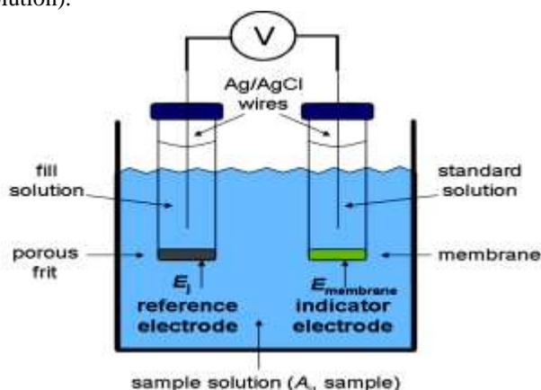
Figure 1: Representation of an electrochemical cell for the measurement of potential.
