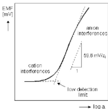
Figure. 2 Typical calibration curve of an ion-selective electrode
