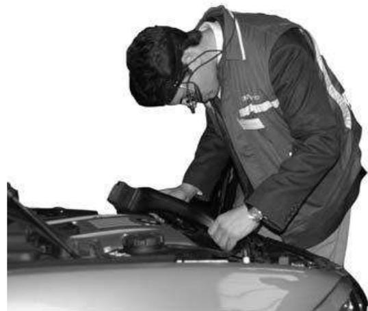
Fig. - 13. Optical see-through HMD used in the maintenance procedure of a commercial vehicle.
