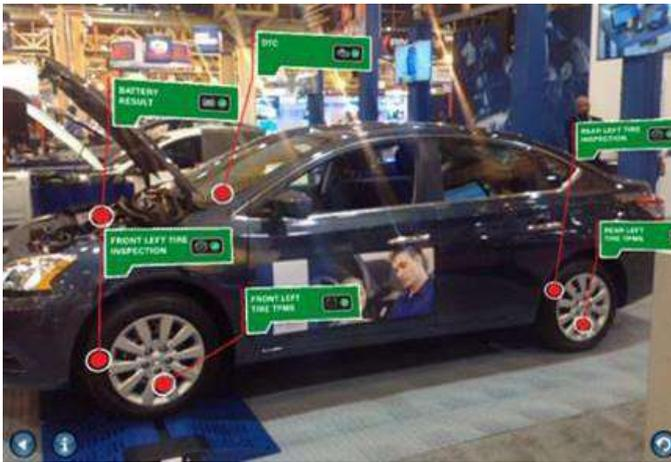
Fig. -14 AR diagnostic system used in car workshops. The worker points his tablet at the vehicle and receives an immediate diagnosis of the major systems in real-time.
