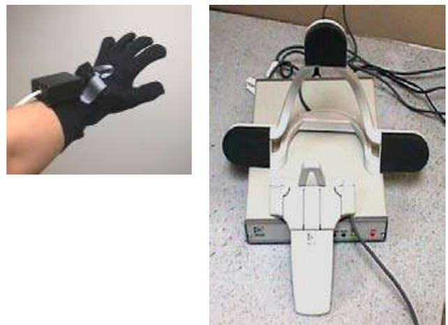
Fig – 4 (a) data glove - 5th Glove<sup>TM</sup> (b) 3-D mouse –Logitech
