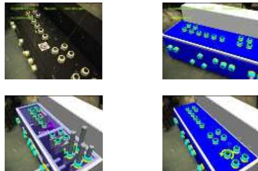
Fig. - 6 Screenshot s of a maintenance procedure on an electrical transformer of a train (a) retrieving name of transformer's parts; (b) animations illustrating a maintenance step.
