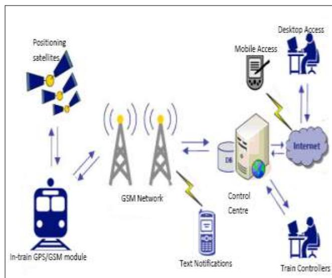
Fig. .1 High Level Architecture
