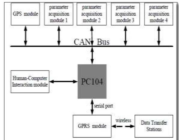
Fig 3. Diagnosis Unit hardware structure
