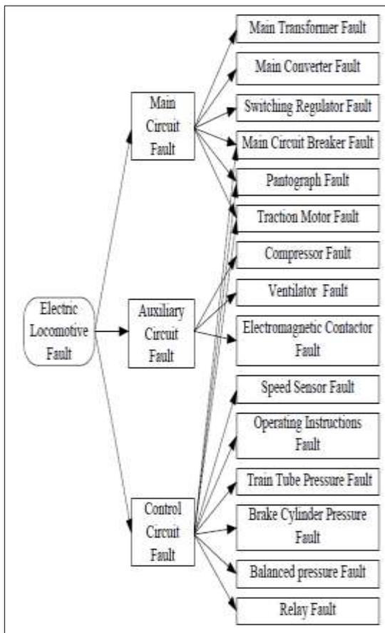
Fig 8. Electrical system faults type of electric locomotive
