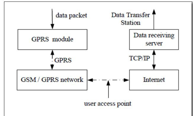
Fig 5.GPRS communication modules
