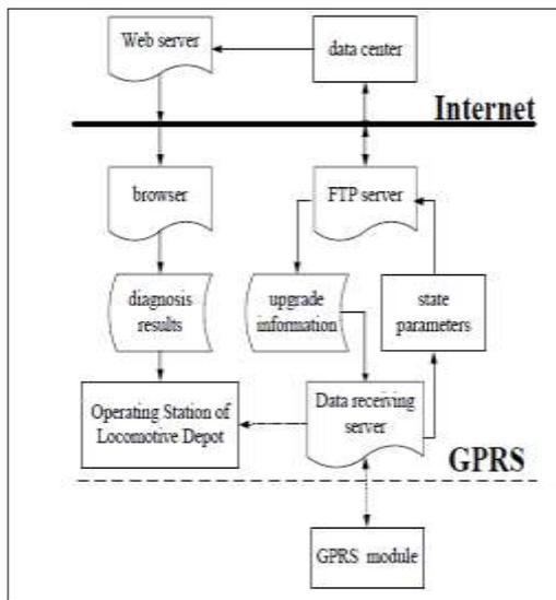
Fig 6. Data Transfer Station block structure
