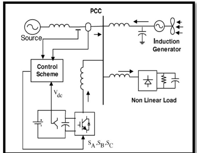
Fig. 5 System operational scheme in grid system Wind Power Generation Model
