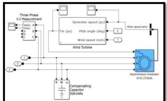
Fig.6 Wind Generating System Model
