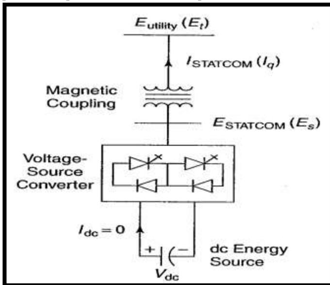
Fig.2 Single Line Diagram of STATCOM
