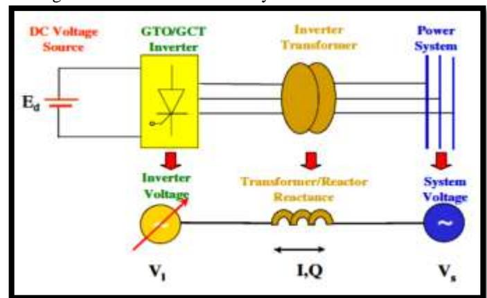
Fig. 1 STATCOM arrangement in power system
