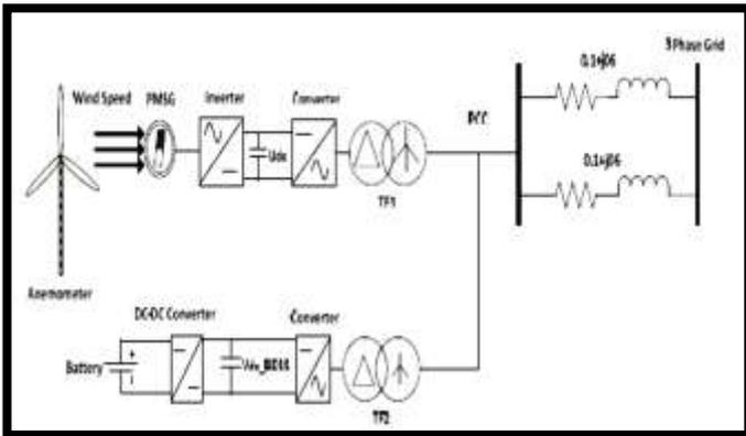
Fig. 3 BESS Configuration with Converter
