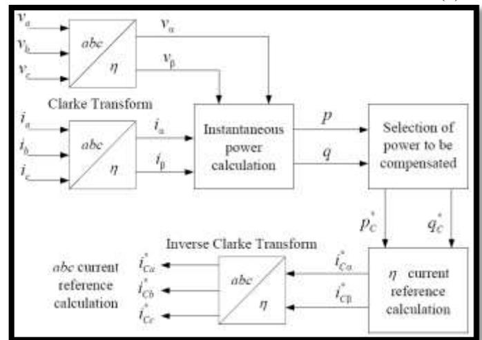
Fig. 4. Control block of shunt current compensation based on the instantaneous power theory
