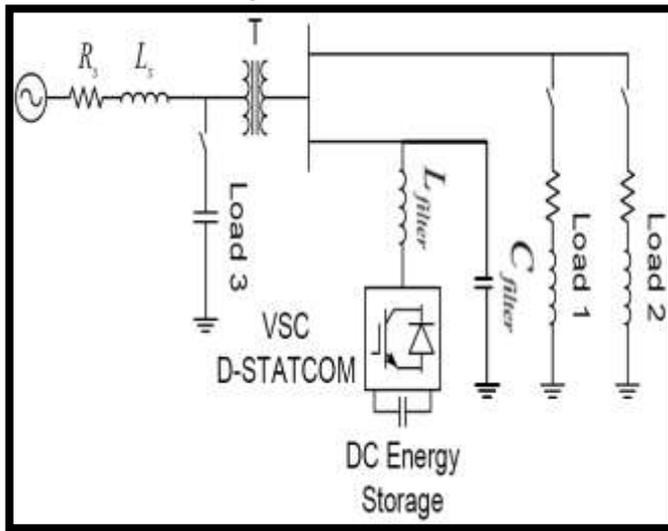
Fig-3 Simplified power system equipped with a D-STATCOM
