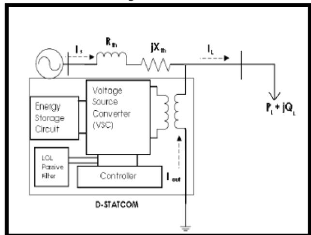
Figure: 1 Schematic diagram of a DSTATCOM
