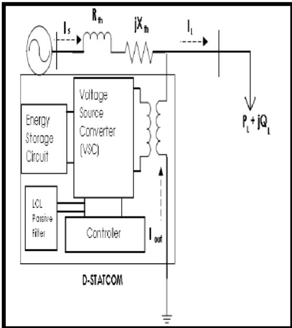
Fig 3: System scheme for d-statcom
