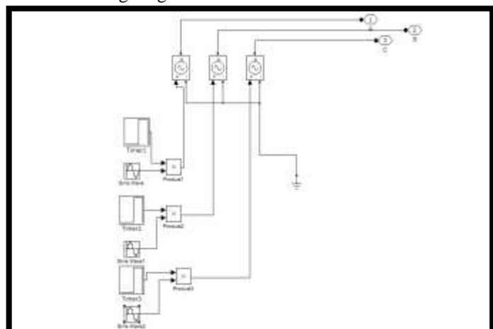
Fig 10- Three phase power supply with external timer signal control
