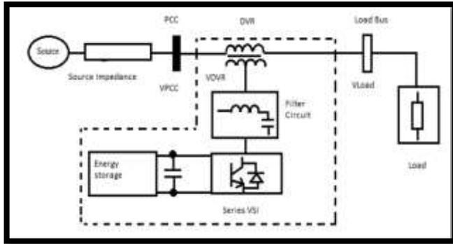
Figure 1 DVR series connected topology
