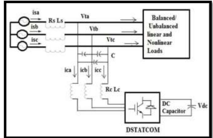
Fig-2: Schematic Diagram of DSTATCOM
