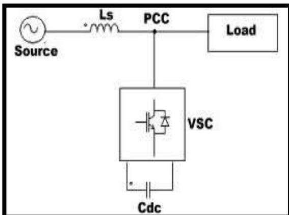
Fig 4: Basic structure of d-statcom
