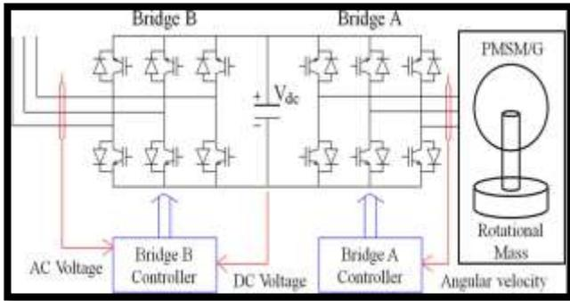
Fig. 2 Grid connection diagram of 900 kW PMSM/G
