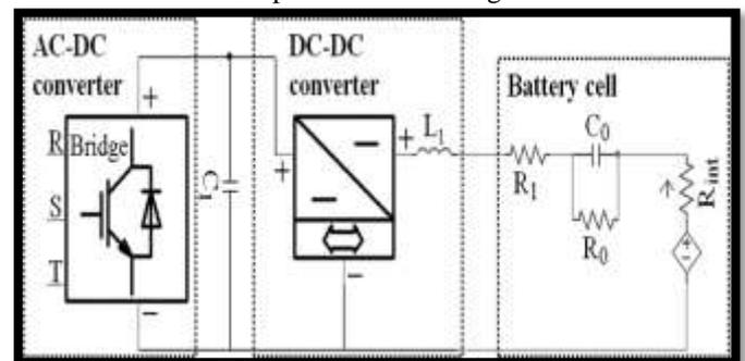
Fig. 1 Battery model and controller set
