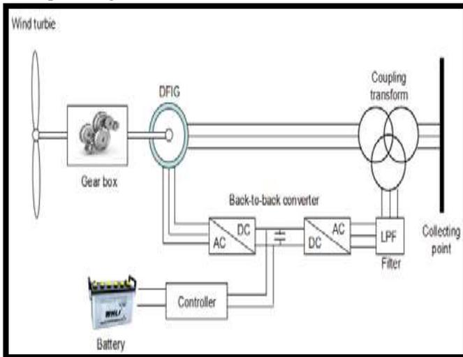
Fig. 3 BESS integration with wind energy conversion system
