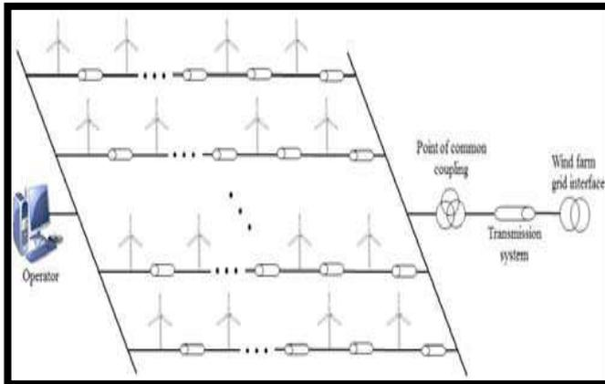
Fig. 4 The network layout of the wind farm
