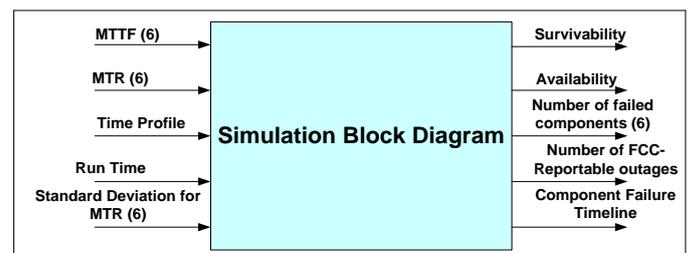
Figure 3: Simulation Block Diagram
