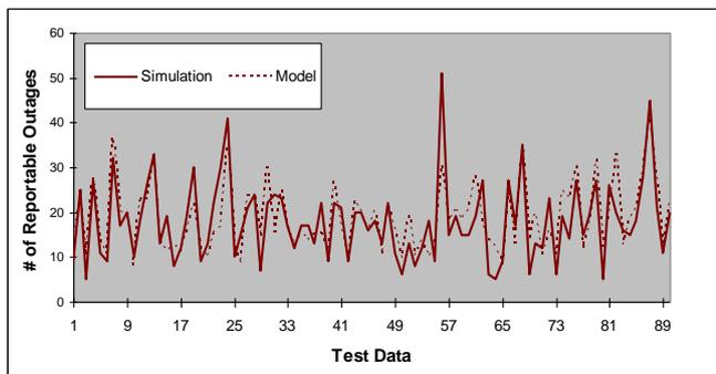
Figure 6: Actual versus NN Output for test data
