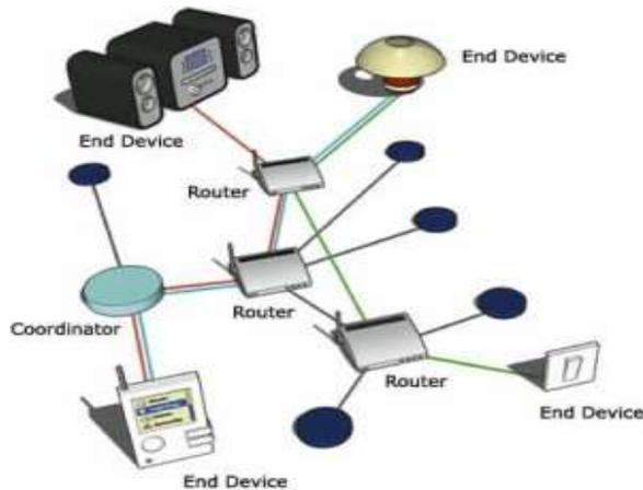
Figure-1 Zigbee Communication Operation
