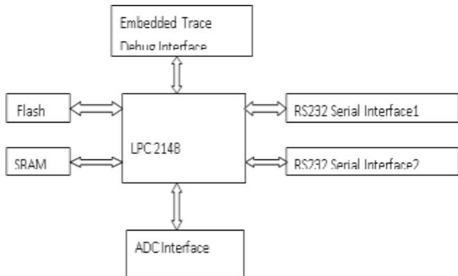
Figure 3.The Hardware Structure of Processing Terminal.
