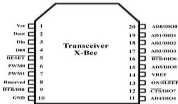
Figure 6. Pin Diagram of Zigbee Transceiver
