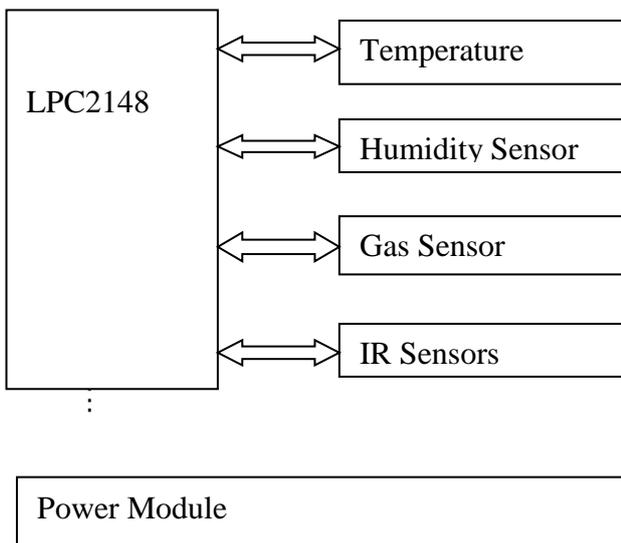
Figure 4 .Hardware Structure of Sensor node.
