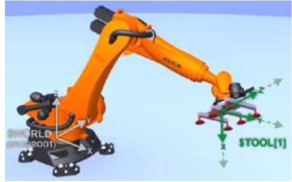
FIG.9: TOOL COORDINATE SYSTEM
