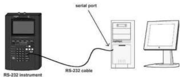
Fig5. System RS-232 instrument connected to computer via serial port
